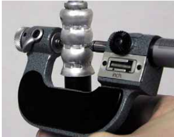
Figure 1 Measuring the crimp with a micrometer.
